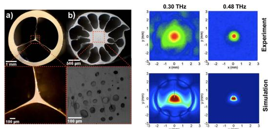
Figure 0.4: Sub-wavelength sized, solid-core fibers used for transport of electromagnetic radiation and THz near-field images at the fiber exit. [25]
