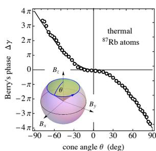
Figure 0.1: Observation of Berry's geometric phase which is imprinted in quantum superposition states of Rb-atoms by rotating the laboratory magnetic field at a cone angle  $\theta$  [3].
