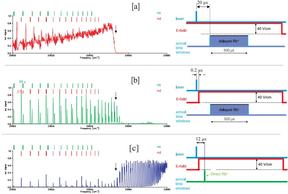
**Figure 1:** Rydberg spectra of *Rb* atoms loaded in a MOT measured with three different timing schemes. Vertical arrow marks the field ionization threshold.
