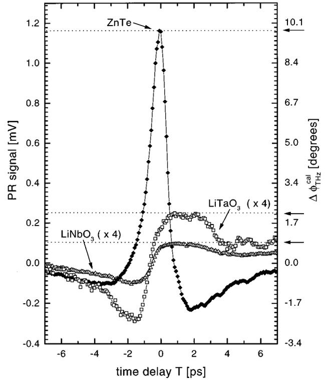
FIG. 2. The left y axis indicates PR signal measured with ZnTe (filled diamonds), *b*-cut LiTaO<sub>3</sub> (open squares), and *c*-cut LiNbO<sub>3</sub> (open triangles). The signals measured with LiTaO<sub>3</sub> and LiNbO<sub>3</sub> are multiplied by a factor of 4. The arrows on the right y axis label the values of the peak PR signals  $\Delta\phi_{\text{THz}}^{\text{cal}}$  calculated from Eq. (5) for different eo crystals used.
