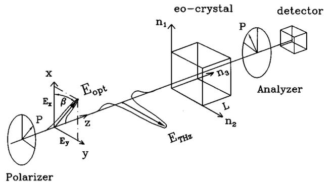
FIG. 1. eo detection setup. The optical probe pulse and the THz pulse propagate along the  $z$  axis. The optical probe beam is linearly polarized at  $\beta = 45^\circ$  and the THz field strength  $E_{\text{THz}}$  is parallel to the  $y$  axis. For  $b$ -cut crystals the following conditions hold:  $n_o = n_1 = n_3$  and  $n_e = n_2$ . For a  $c$ -cut crystal:  $n_o = n_1 = n_2$  and  $n_e = n_3$ .
