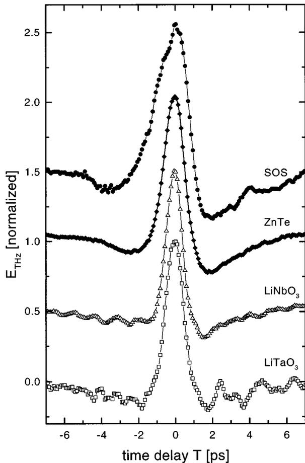
FIG. 4. The electrical THz field strength  $E_{\text{THz}}$  measured with LiTaO<sub>3</sub> (*b*-cut), LiNbO<sub>3</sub> (*c*-cut), ZnTe and with a SOS detector. The vertical zero is offset for each trace by 0.5. The SOS detector is slower compared to the eo detection mechanism, because of imperfect focusing of the optical gate pulse onto the detector gap.
