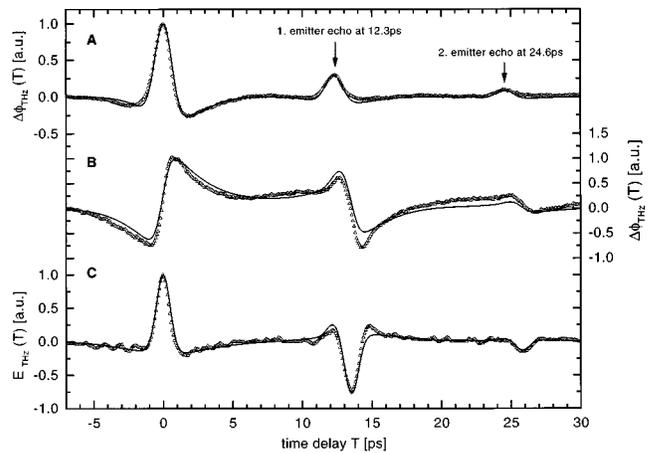
FIG. 3. Trace A: normalized PR signal measured with ZnTe. Multi étalon THz echos at  $T = 12.3$  ps and  $T = 24.6$  ps from the GaAs emitter are well resolved. The thin solid lines represent the calculated data using Eq. (5). Trace B: normalized PR signal measured with *c*-cut LiNbO<sub>3</sub> as sensing crystal. Trace C: differentiated trace B giving  $E_{\text{THz}}(T)$ .
