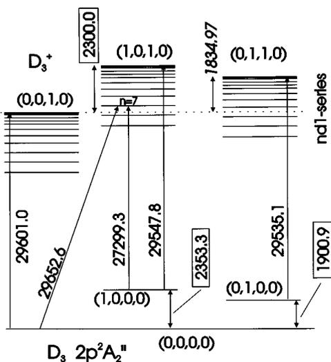
FIG. 6. Energy level scheme of the  $D_3$  and  $D_3^+$  molecule states relevant for the data presented in this paper. Observed transitions are indicated by single-arrow lines and labelled by the transition frequencies in cm<sup>-1</sup>. The degenerate mode spacing of  $D_3^+$  given in italics is calculated from the molecular constants by Amano *et al.*<sup>35</sup> The vibrational spacings deferred from the experimental results are enclosed in boxes.
