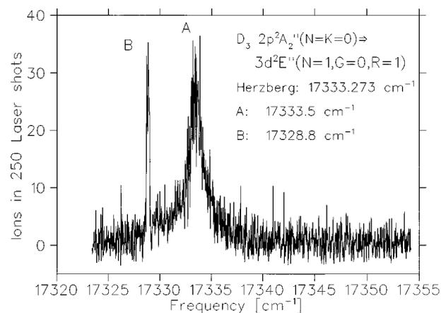
FIG. 2. Two-photon ionization spectrum of metastable  $D_3$  molecules in the  $17320\text{ cm}^{-1}$  to  $17355\text{ cm}^{-1}$  photon energy range. Peak A is due to the  $2p\ ^2A''_2(N=K=0) \rightarrow 3d\ ^2E''(N=1, G=0, R=1)$  transition observed in emission at  $17333.273\text{ cm}^{-1}$  by Herzberg *et al.*<sup>4</sup>
