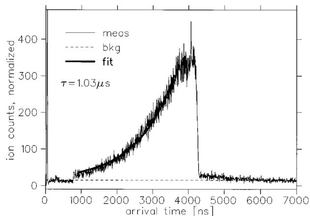
FIG. 7. Arrival time spectrum of the photoions with the laser exciting the transition from the  $D_3 2p \ ^2A_2''(N=K=0)$  state into the continuum. The laser beam was expanded and collimated in order to produce a homogeneous beam profile over the entire length of the interaction region. The solid line is a single exponential fit to the measured spectrum between 900 ns and 3600 ns with a lifetime of  $\tau=1.03 \mu\text{s}$ .
