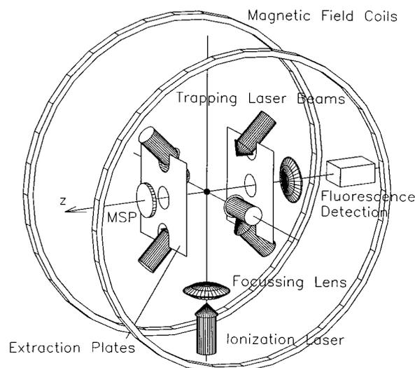
FIG. 1. Schematic of the ion recoil spectrometer with laser-cooled target. Atoms in a standard MOT are ionized by a pulsed laser. The ions are extracted by a weak electric field along the  $z$  axis.
