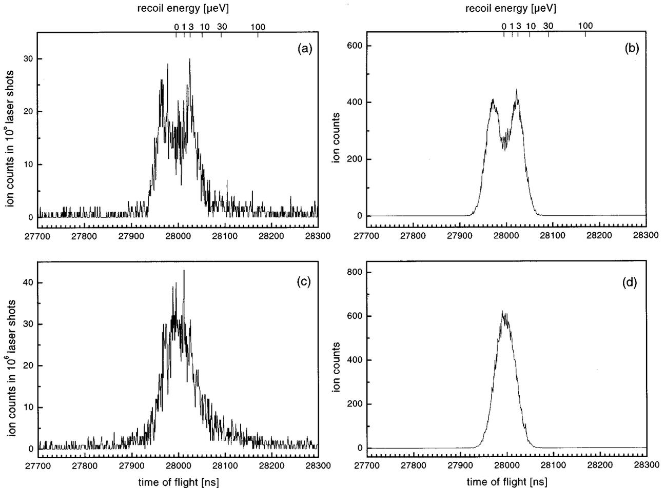
FIG. 2. Experimental time-of-flight spectra of  $\text{Rb}^+$  ions with laser polarization (a) parallel and (c) perpendicular to the extraction field. The laser pulse energy was approximately 20 pJ. Monte Carlo simulations of the time-of-flight spectra are shown in (b) and (d) with parameters for (a) and (c), respectively.
