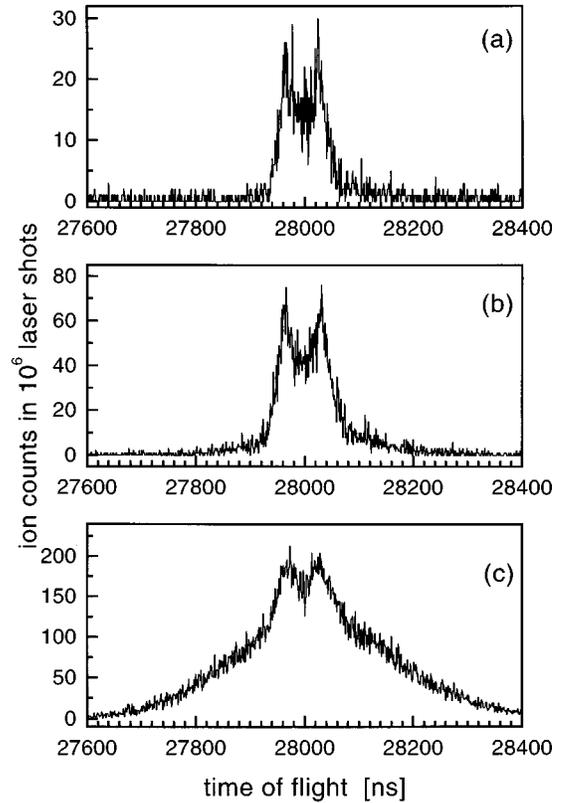
FIG. 4. Experimental time-of-flight spectra for different pulse energies,  $E_{\text{pulse}}$ , of the ionization laser: (a)  $E_{\text{pulse}} \approx 30 \text{ pJ}$ , (b)  $E_{\text{pulse}} \approx 20 \text{ pJ}$ , (c)  $E_{\text{pulse}} \approx 60 \text{ pJ}$ .
