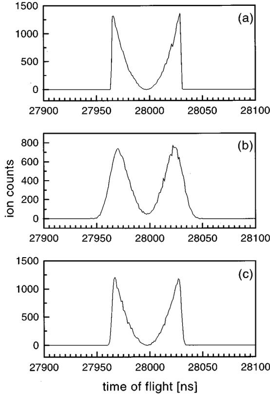
FIG. 3. Monte Carlo simulations of time-of-flight spectra of  $\text{Rb}^+$  ions for idealized and realistic experimental parameters: (a) trap temperature  $1 \mu\text{K}$ , laser beam waist  $1 \mu\text{m}$ ; (b) trap temperature  $1 \mu\text{K}$ , laser beam waist  $20 \mu\text{m}$ ; (c) trap temperature  $150 \mu\text{K}$ , laser beam waist  $1 \mu\text{m}$ .
