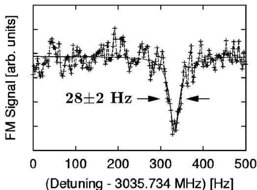
FIG. 6. Dark resonance signal observed at  $I_0 = 300 \text{ nW/cm}^2$  using the large-diameter beam (the peak corresponds to the resonance at  $\omega_{\text{DR}}/2\pi + f_{\text{mod}}$ ).
