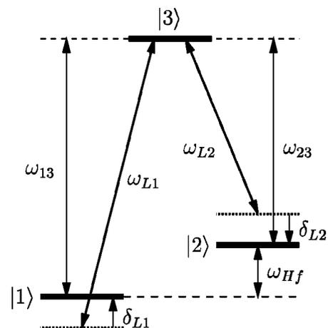
FIG. 1. Notation of the frequencies of the  $\Lambda$  scheme. In our experiments on  $^{85}$ Rb the labels  $|1\rangle$ ,  $|2\rangle$ , and  $|3\rangle$  refer to the states  $|^2S_{1/2}, F=2, m_F=0\rangle$ ,  $|^2S_{1/2,3,0}\rangle$ , and  $|^2P_{3/2,3,\pm 1}\rangle$ , respectively.
