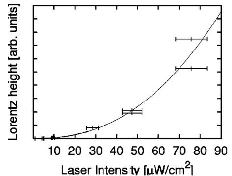
FIG. 5. Dependence of the dark resonance height on laser intensity for  $^{85}\text{Rb}$  (small-diameter beam).
