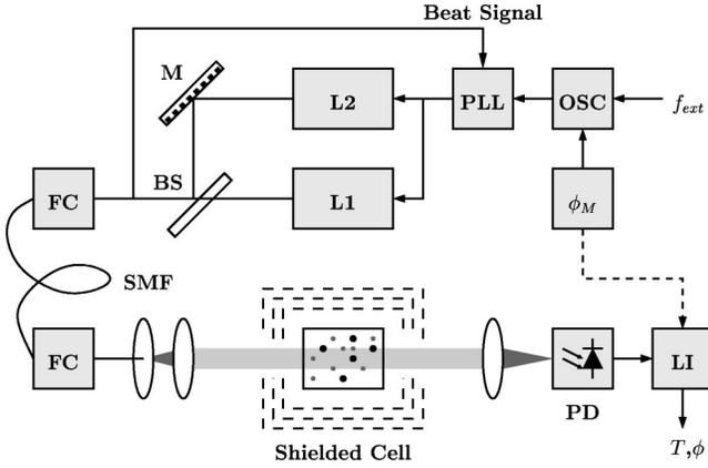
FIG. 2. Schematic of the experimental setup. Two external-cavity diode lasers (L1 and L2) are phase-locked (PLL). The modulated ( $\Phi_M$ ) oscillator (OSC) is externally tuned ( $f_{\text{ext}}$ ) while a lock-in amplifier (LI) monitors the transmitted intensity (M, mirror; BS, beam splitter; FC, fiber coupler; SMF, single-mode fiber).
