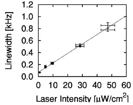
FIG. 4. Dependence of the dark resonance width on laser intensity for  $^{85}\text{Rb}$  (small-diameter beam).
