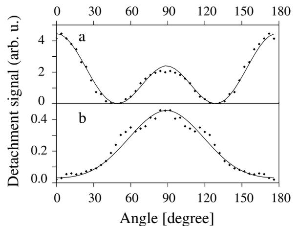
FIG. 5. Angular distributions of photoelectrons in the lowest two-photon detachment channel at two different laser intensities: (a)  $I = 1.3 \times 10^{11}$  W/cm<sup>2</sup>, (b)  $I = 6.5 \times 10^{11}$  W/cm<sup>2</sup>. Experimental data (dots) and theoretical results (solid curves) are normalized to each other.
