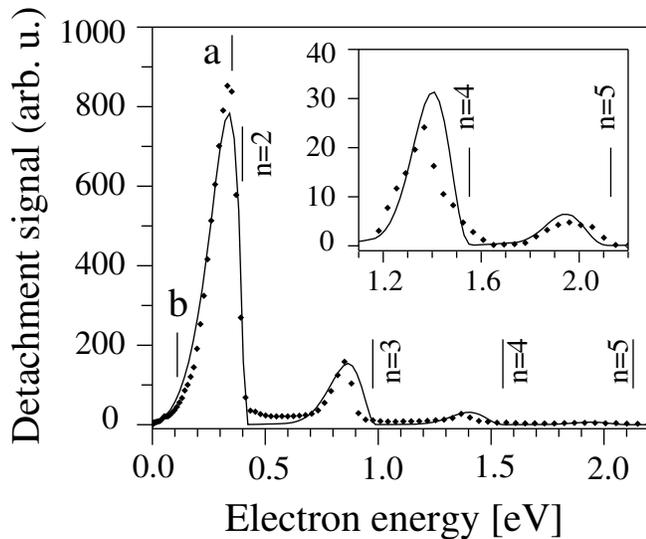
FIG. 4. The energy spectrum integrated over the angle  $\theta$ : dots—experimental data; solid curve—theoretical results. Angular distributions at energies labeled  $a$  and  $b$  are shown in Fig. 5. The inset shows higher energy peaks in a greater detail.
