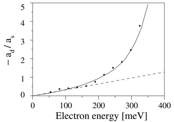
FIG. 6. The amplitude ratio of the  $d$  and  $s$  waves near the threshold of photodetachment. Dots—experimental results; solid curve—theoretical prediction. Notice that the amplitudes have opposite signs. The dashed line shows the linear dependence according to the Wigner threshold law.
