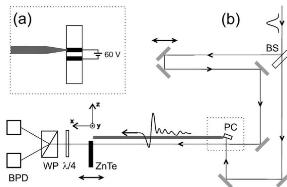
FIG. 1. (a) Side view of the photoconductive emitter with the wire tip contacting the positive electrode. (b) The experimental setup. (BS=beam splitter, PC=photoconductive switch emitter, WP=Wollaston polarizer, BPD=balanced photodiodes.)
