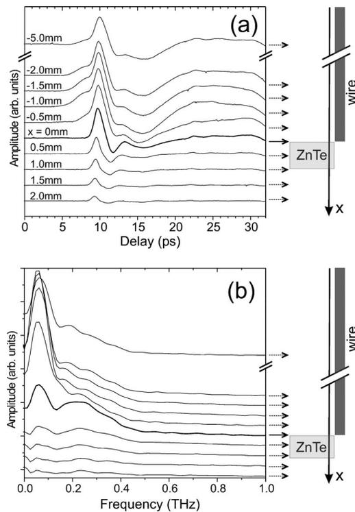
FIG. 2. (a) THz pulses measured at different positions along the metal wire axis. (b) Corresponding frequency spectra of the THz pulses in (a). The collimation of the 800 nm sampling beam, which travels alongside the THz pulse parallel to the wire, was optimized for the  $x=0$  position. This may account for slight distortions in the THz wave form at positions  $<0$  in (a).
