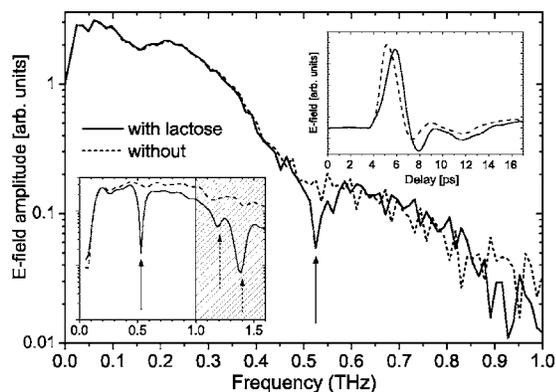
FIG. 4. Frequency spectra of THz pulses propagated along the wire with (solid line) and without lactose powder on the wire (dashed line). The upper inset shows the corresponding THz pulses. The arrow indicates a distinct absorption of lactose at 0.53 THz. The lower inset shows THz transmission spectra of lactose recorded with a conventional THz-TDS setup. The arrows indicate absorption bands of lactose.
