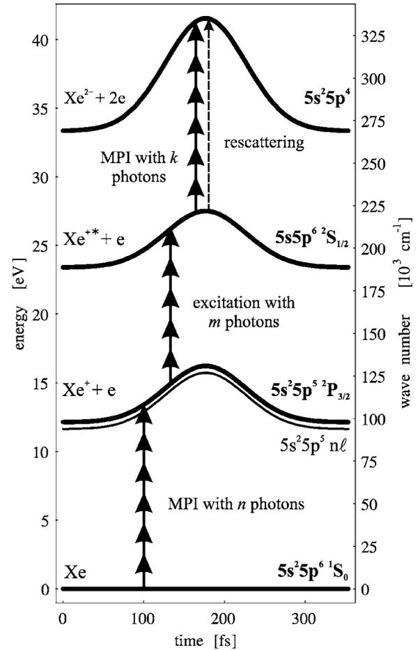
FIG. 2. Schematics of the proposed double ionization mechanism of xenon atoms based on resonance enhancement by the ionic transition and a two-electron transition involving the rescattered electron. The graph is drawn for a laser pulse with a peak intensity of  $3 \times 10^{13} \text{ W}/\text{cm}^2$  and a wavelength of 1200 nm. The excited states and continua follow the temporal development of the laser intensity.
