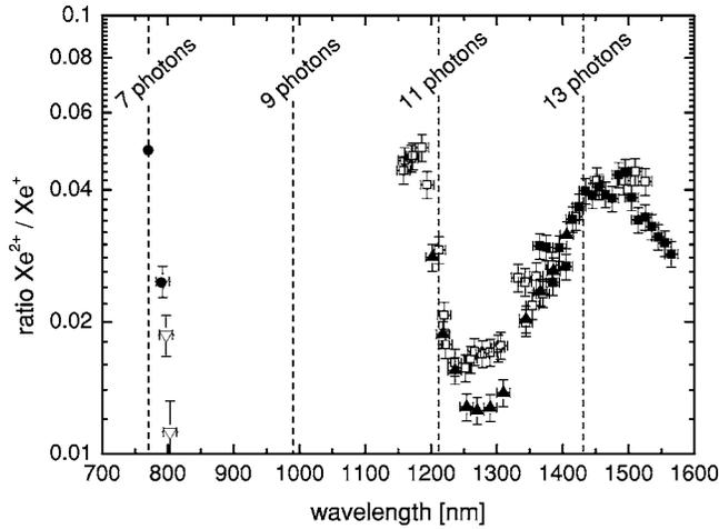
FIG. 1. The ratio of doubly to singly charged xenon ions is shown as a function of wavelength for various peak intensities. The peak intensities are  $40.0 \pm 1.9$  (open triangles),  $38.9 \pm 1.9$  (open squares),  $25.2 \pm 1.2$  (solid triangles), and  $21.8 \pm 1.1$  (solid squares)  $\text{TW}/\text{cm}^2$ . The ratio for 790 and 770 nm measured by Rudati *et al.* [13] at an intensity of  $40 \text{ TW}/\text{cm}^2$  (multiplied by a factor of 4.1) is shown by the solid circles.
