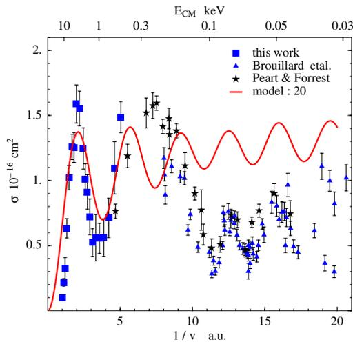
FIG. 5 (color online). Predicted cross section (divided by a factor of 20) based on the ion-pair splitting labeled *model* in Fig. 3.
