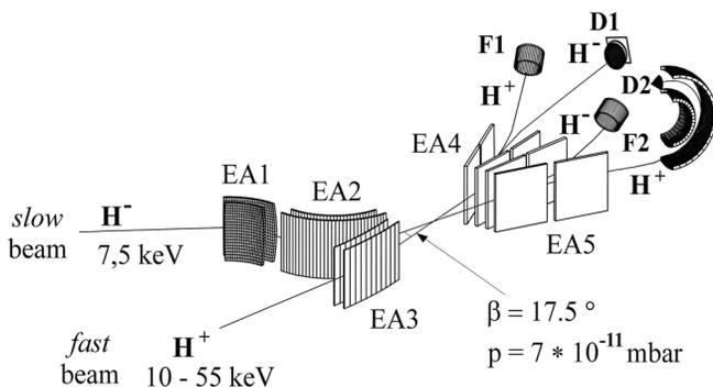
FIG. 1. Schematic overview of the Giessen ion-ion experiment. EA1-EA5: electrostatic analyzers, F1, F2: Faraday cups, D1: microchannel plates, D2: channeltron detector.
