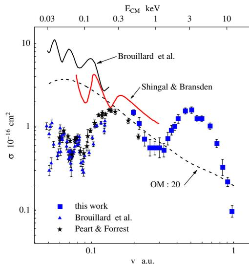
FIG. 2 (color online). Total cross sections for the reaction  $H_a^- + H_b^+ \rightarrow H_a^+ + H_b^-$ . Error bars represent the statistical error only for the three experimental data sets. Also included are the predictions by Shingal and Bransden [7] and by Brouillard *et al.* [3]. OM is the prediction of Eq. (1), based on the splitting of the ionic diabatic states of O'Malley [9] (stars in Fig. 3).
