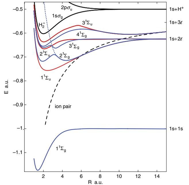
FIG. 4 (color online). Potential energy curves of the lowest states of  $H_2$  and  $H_2^+$ , taken from Refs. [13,14]. The curves shown in blue are of  $1^1\Sigma_g$  character, those in red of  $1^1\Sigma_u$  character. State labels for 1, 2,  $3^1\Sigma_u$  are  $B, B', B''$  and for 1, 2, 3,  $4^1\Sigma_g$  they are  $X, EF, GK, H\bar{H}$ . The short dashed line gives the diabatic 2,  $3^1\Sigma_g$  state. The long dashed line is the attractive Coulomb curve.
