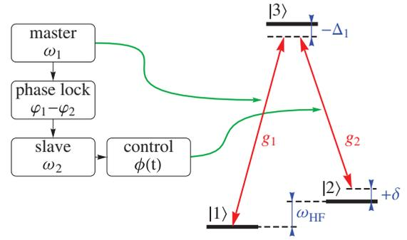
FIG. 1. (Color online) Scheme of experimental frequency and phase control using the simplified  $\Lambda$  system.
